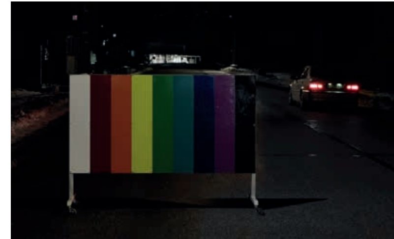
HME – road and environs have a blue-green tinge. Color rendering is limited. R_a 45-60
