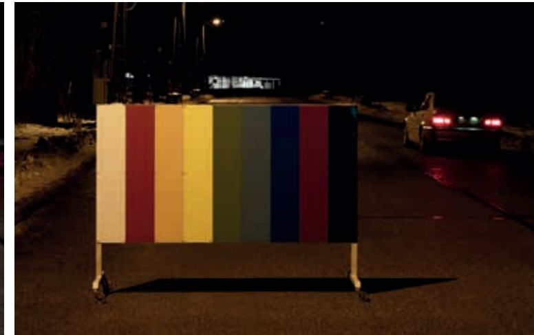
HST – road and surroundings have a yellow tinge. Color rendering is poor. R_a \leq 25
